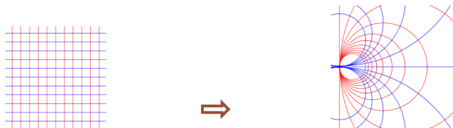
Figure: x^\mu \rightarrow \frac{x^\mu - a^\mu x^2}{1 - 2a \cdot x + a^2 x^2} transformation
